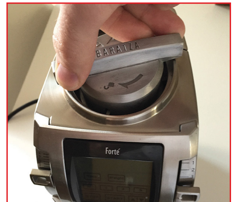
Turn burr clockwise to remove
